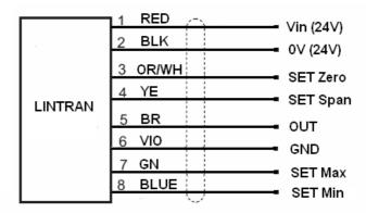
'Set Max' and 'Set Min' are factory settings and should not be connected without prior consultation with Zettlex.
